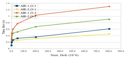
Weak scalability (up to 16384 cores) of pAIR (with AMG restriction distance 1 and 2) for DG advection problem. Standard AMG, if combined with GMRES, can only solve the two smallest problems, but is much (~4x,~8x) slower.
